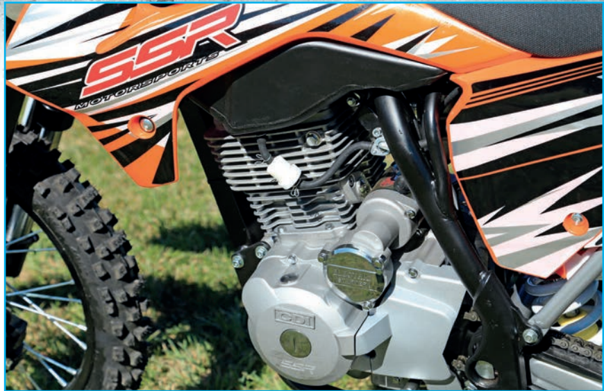
The SSR 150's motor is a happy revver, but it runs well down low. There is a giant air filter element under the side plastic.
