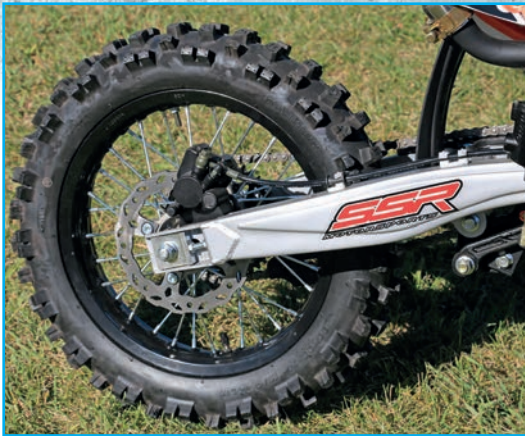
The swingarm looks aluminum, but it is steel. The hubs look large enough for a full-size bike.
