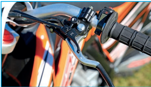
It is nice to have the choke right where you can get at it easily. The clutch must be pulled in before the bike will start.
