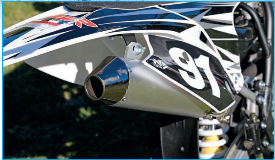
This muffler looks suspiciously like a KTM two-stroke muffler, and the sound is reasonable, but no spark arrestor is a problem.
